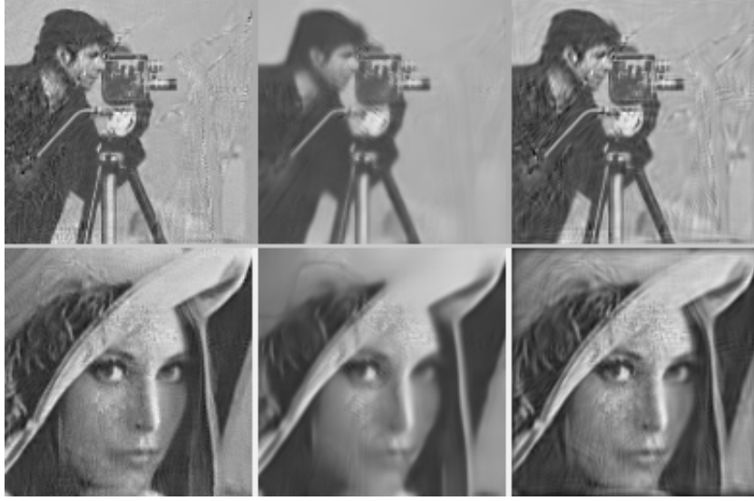
Figure 9: Reconstruction of varying phase (cameraman) and amplitude (Lena): from left-to-right: BM_2 , Sp , WFT algorithms, noisy observations, \sigma = 0.1 .
