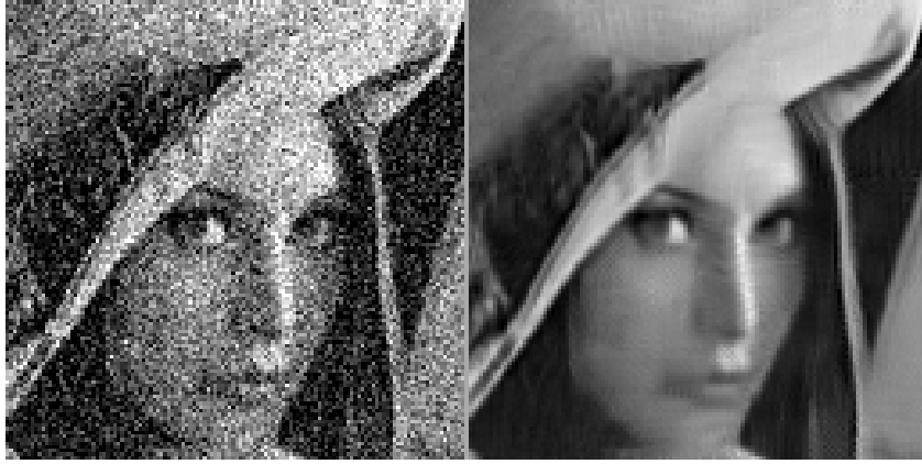
Figure 7: Lena phase images: noisy phase observation (left) and iterative CDBM3D phase reconstruction (right), \sigma = 0.3 . PSNR for the reconstruction is 40.29 dB and for the noisy phase is 29.27 dB.
